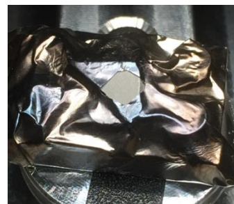
Image of foil with aperture in the center to minimize charging. The sample was AuPd coated after the foil was placed on top.
