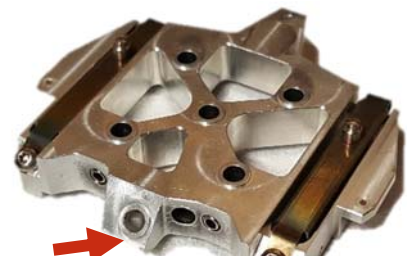
FIGURE 2. USE THE 45 DEGREE PRETILTED END OF THE SHUTTLE HOLDER
