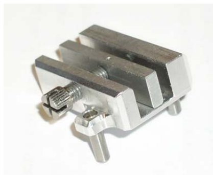
FIGURE 2-5 X-SECTION SAMPLE HOLDER MULTI/STUB SAMPLE HOLDER
