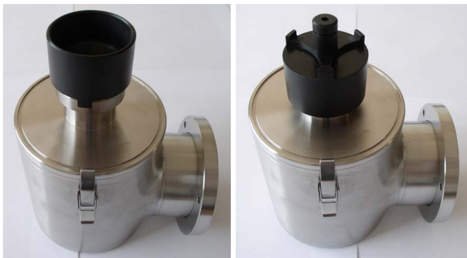
FIGURE 5-22 PLASTIC CAP FILLING POSITION PLASTIC CAP OPERATION POSITION
