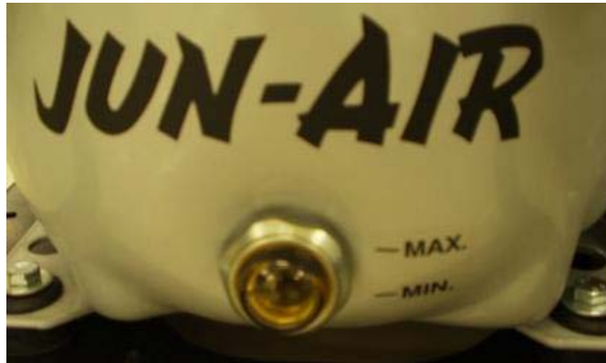
FIGURE 6-1 COMPRESSOR OIL LEVEL CHECK
